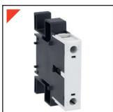
Three-pole contactors for currents from 26 to 150 A can be supplemented with the fourth power pole, which is installed by snapping on and converts a three-pole contactor into the four-pole one.
