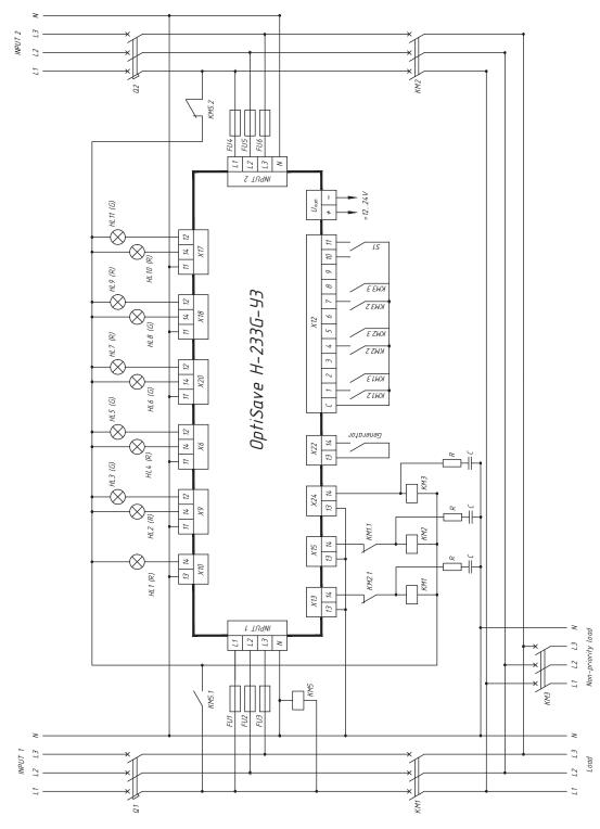
KM1, KM2, KM3 – switching devices (contactors, starters); KM1.1, KM1.2 —contacts for blocking simultaneous switching on of input SDs KM1.2, KM2.2, KM3.2 – signaling contacts of switching devices; KM5 – relays for switching the power supply of external control and signaling
