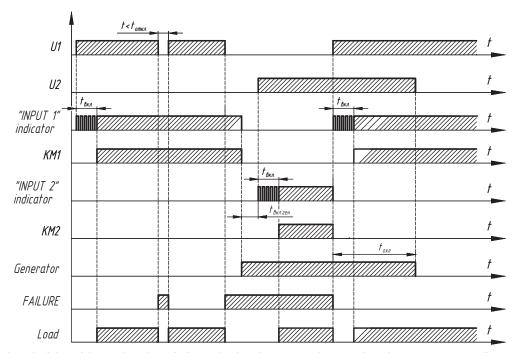
The decision about the failure of the switching device (SD) is made when the SD status changes without the ATSU issuing controlling actions. The ATSU in the automatic mode does not restore the SD's health attribute without the operator's intervention. After the SD failure causes have been eliminated, error reset must be performed in the ATSU menu.
