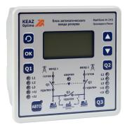
OptiSave H automatic transfer switch unit is designed to build various ATS functional solutions based on contactors, load switches and electromagnetic and motor driven circuit breakers with the option of being integrated into dispatching systems via Modbus protocol.
