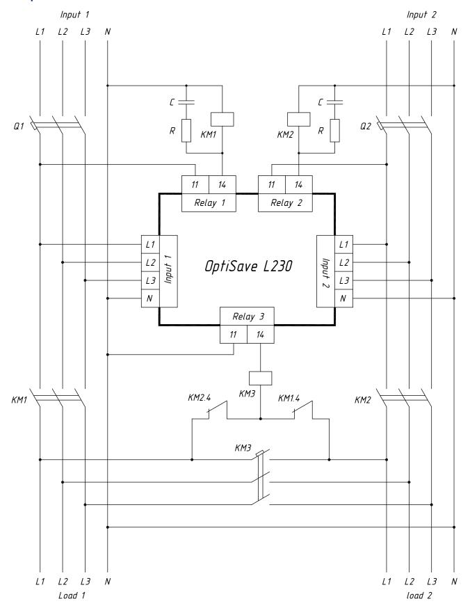
Q1, Q2 – automatic circuit breakers;
