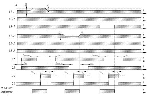
The decision about the failure of the switching device (SD) is made when the SD status changes without the ATSU issuing controlling actions. The ATSU in the automatic mode does not restore the SD's health attribute without the operator's intervention. After the SD failure causes have been eliminated, error reset must be performed in the ATSU menu. In the presence of the "SD Deleted" signal, the ATSU operation algorithm is blocked.
