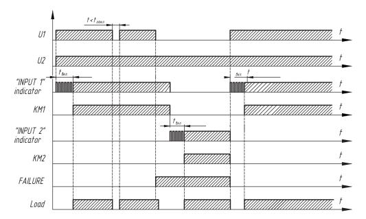
Timing diagram of ATSU operation in AUTO mode with the preset INPUT 2 value of generator using the example of voltage loss on INPUT 1
