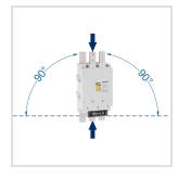
Mounting upright or turning right / left 90°. Power supply from above and below.
