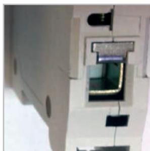
Notches on the terminal clamps provide the most tight contact, increase the mechanical strength of the connection and reduce the value of the transient resistance, thereby ensuring that connected conductors do not overheat and melt.
