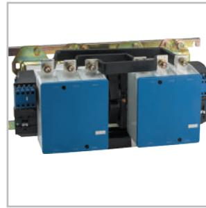
High rigidity of the structure and reduction of mounting errors for contactors with rated currents over 100 A is provided by the presence of a factory connection in the main circuit, installation of contactors on two metal rails and mechanical interlocking.
