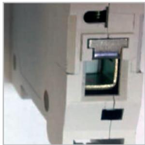
Notches on the terminal clamps provide the most tight contact, increase the mechanical strength of the connection and reduce the value of the transient resistance, thereby ensuring that the connected conductors do not overheat and melt.
