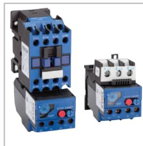
Thermal relays of RTL series can be mounted either directly to the contactor, or separately using the KRL Terminal strip (screws or DIN-rail).
