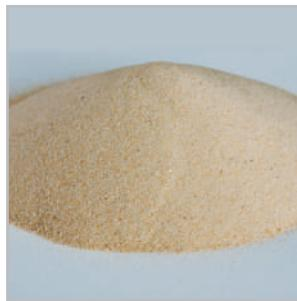
The method of filling the fuses with filler (high purity quartz sand) allows to achieve a high filling density and provides effective damping of the electric arc inside the fuse when it is triggered.
