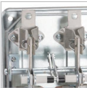
The necessary contact pressure is provided by the springs on the contact racks and spherical washers on the hinge racks.
