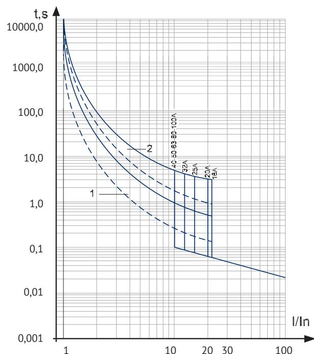
1 — working zone of an overcurrent thermal release, measured in hot state
