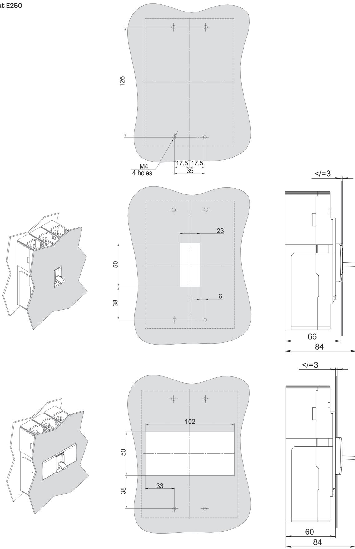
► Installation versions of rotary remote handle OptiMat E100 and E250
