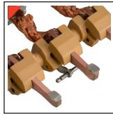
The use of modern materials: silver-containing contacts reduce transient resistances, increase welding wear resistance and exclude welding susceptibility; non-combustible plastic with improved electrical insulation properties and arc resistance.
