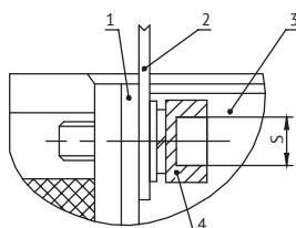
Cable connection without wiring terminal connector
