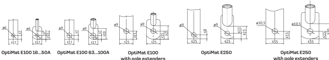
Minimum allowable distance from OptiMat E100 and E250 switches to metal parts of switchgear
