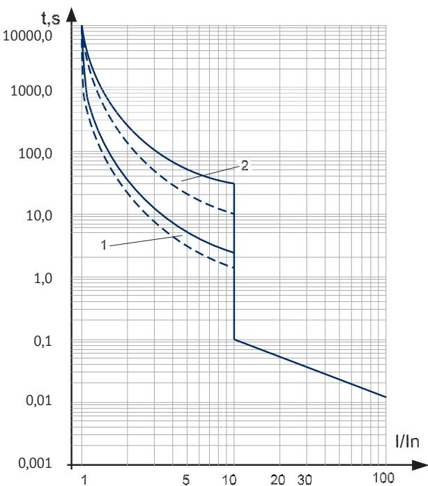
1 — working zone of an overcurrent thermal release, measured in hot state
